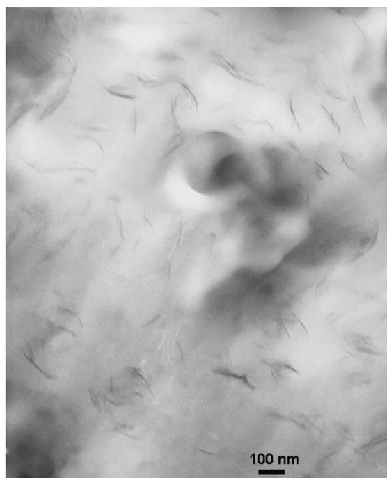
Fig. 3. The TEM images of ABS/10A-clay nanocomposite having 3.0% inorganic clay content at low magnification (left, 10,000 \times ) and high magnification (right, 50,000 \times ).
